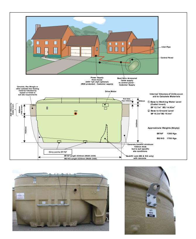
5.10 BG and NG BioDisc have an off-set centre of gravity and should not be lifted by the base channels as this would risk tipping over the unit. The old slinging points are still in the bottom of the mould, they are not to be used under any circumstances. Lift using the 4 new metal lifting brackets as indicated by labels on the unit.
